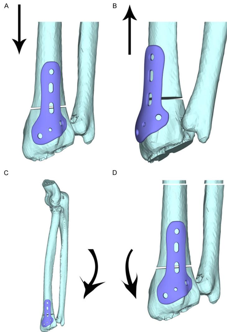
**Figure 3.** Force condition of AO non-bridge distal radius fracture model under all operating conditions. A: Under the operating condition of contraction; B: Under the operating condition of stretching; C: Under the operating condition of internal rotation; D: Under the operating condition of external rotation.
