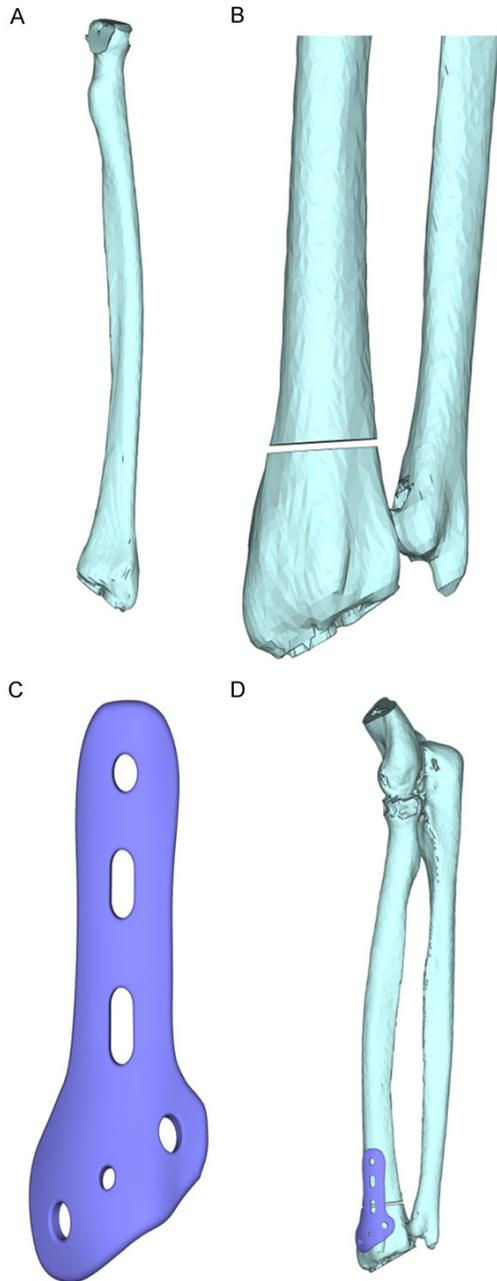
**Figure 1.** Three-dimensional stereo model after non-bridge external fixation of distal radius fracture. A: Radius three-dimensional visualization model; B: Distal radius fracture model; C: AO non-bridge external fixation model; D: Distal radius fracture model equipped with AO non-bridge external fixation.
