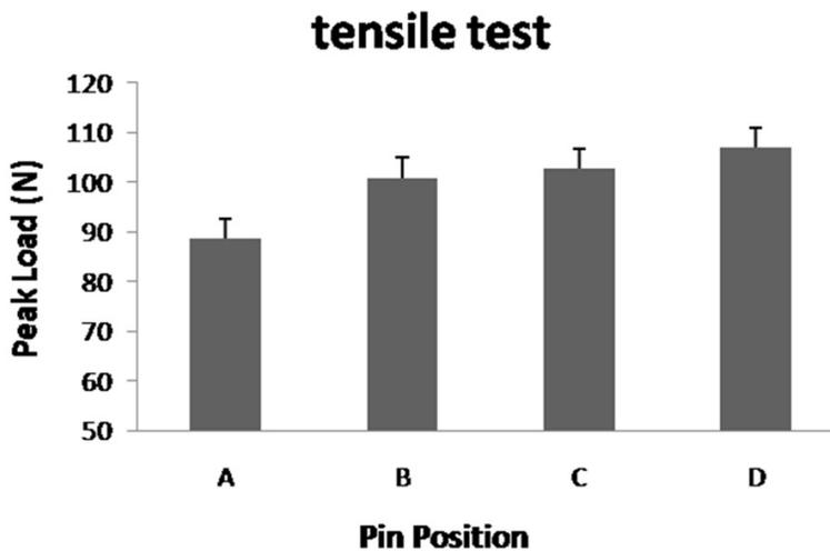
**Figure 5.** Comparison of the peak loads on different pin positions in the tensile test. Compared with the other three groups, group D showed the highest fixation stability effect at peak load.
