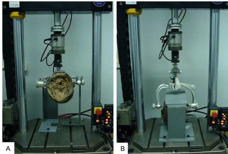
**Figure 3.** Biomechanical test with the base unit of the electromagnetic motion analysis device. A. Skull in the compression test; B. Skull in the tensile test.
