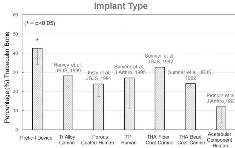
**Figure 5.** Porous ingrowth. Percentage of ingrowth-bone contact on the endplate surface. The bar graph illustrates porous ingrowth for the novel disc prosthesis that is more favorable than that reported for total joint arthroplasty in the peripheral skeleton.
