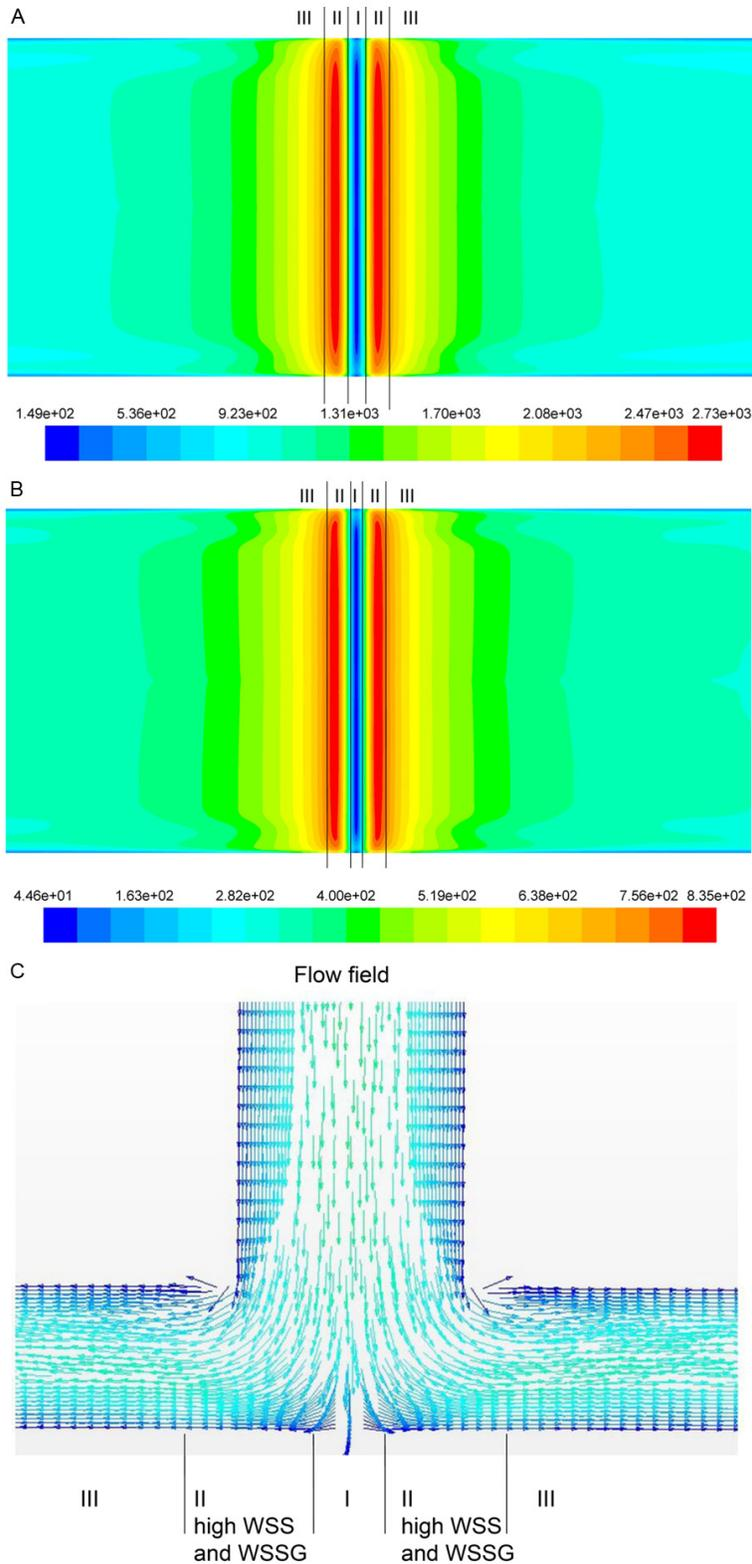
**Figure 2.** A. CFD simulation of WSS and WSSG of the impinging flow in the flow rate of 250 ml/min; B. CFD simulation of WSS and WSSG of the impinging flow in the flow rate of 500 ml/min; C. CFD stimulation for 2D geometry at the rate of 250 ml/min; Three flow zone, velocity magnitude and direction in the T chamber were shown in this image.
