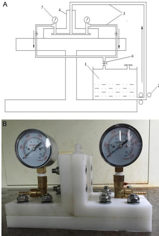
**Figure 1.** A. The map of the T chamber system: the chamber system, 1 reservoir, 2 pump, 3 tube, 4 the T-shape chamber, 5 pressure gauges, 6 flow constrictors; B. The T chamber.
