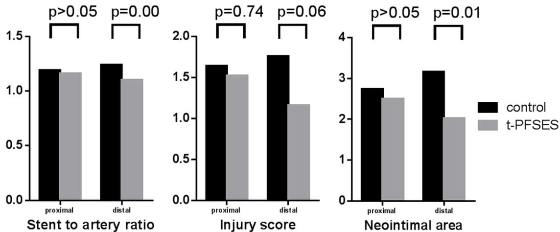
Figure 10. The stent to artery ratio, injury score, neointimal area for control stents and the t-PFSES stents.
